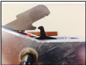
This is the correct reset. The disconnect distance is correct and space is available for reset.
