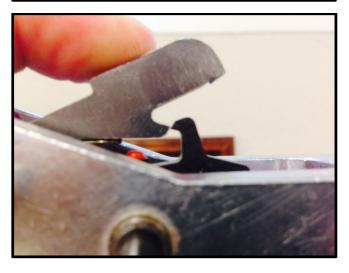
When the bolt carrier resets the hammer the hooks are extremely close but never actually make contact. They should never touch unless you do not release the trigger.
