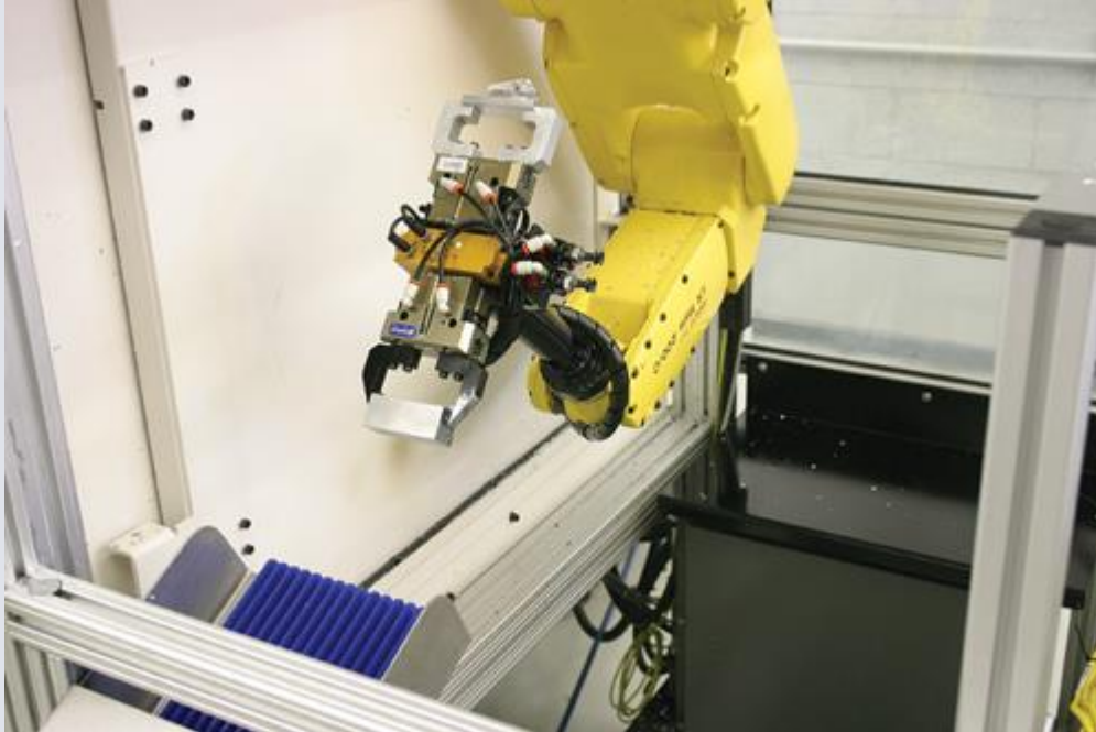
Close up of the robot in a Fanuc RoboDrill getting ready to drop a completed part into the unload chute.
