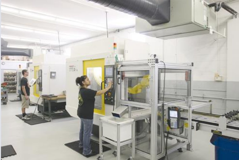
Machine operator Karla Marin prepares to set up one of Timney's three Fanuc Robodrills. Two of the RoboDrills are 5-axis machines equipped with robot loaders. The third, shown in the background, is a 3-axis with a 4th-axis table. Parts are loaded on custom 6-sided tombstones.
