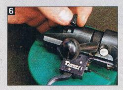
the rifle, including installing the bolt, and check the function of the trigger and the safety. Make sure the safety will go on and that it is working in both the "on" and center positions. Once in a while the safety will not work, which requires the bolt be disassembled and a bit of clearance be cut with a file. Timney can provide instructions on how to do this
