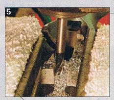
ance in the stock for all the screws and other parts of the trigger. Make sure the retaining screw is not hitting the aluminum bedding block on the stock or it will prevent the action from seating properly. During this Rx installment, I needed to use a milling machine to remove some metal and provide clearance for the trigger screw. Drilling it out with a drill press or even using a Dremel tool to remove the metal would have also worked.
