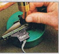
3 IN WITH THE NEW: Slide the new trigger into place, pushing back on the bolt stop spring and stretching it enough that the trigger can be inserted and the rear pin pushed into place to hold it.
