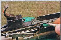
SECURE IT: Tighten the front screw on the trigger until it's snug. This screw is designed to place tension on the locking pins and to remove any movement in the trigger.
