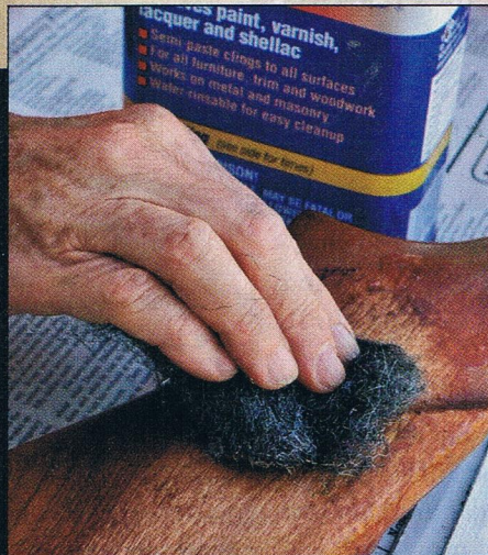
Coarse steel wool and a strong stripping agent rid the stock of old finish and dirt in the pores. Wayne likes the Miles Gilbert stock finishing kit
