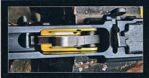
3 CLEAN & REPLACE: Remove all the trigger parts and the safety lever, which is sometimes called the fire control selector. Clean the receiver with a degreasing spray to remove debris.
