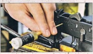
2 PUNCH OUT: It's much easier to work if the gun is held solidly in place, so place a lower receiver vise block into the magazine well and clamp it into your bench vise. Push out the two pins holding the trigger parts in place using a straight punch.
