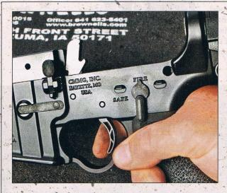
5 TEST IT: Check that the trigger is functioning properly by cocking it and pulling the trigger several times. I like to use a hammer drop block when dry-firing. This is a handy tool if you are doing a lot of this work. If this is a one-time deal, you can get by without it by catching the hammer on your finger.
