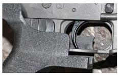
The Slide Fire stock slips back and forth within these limits. Your finger placed in front of the trigger will trip it as you shove forward on the forend. Recoil resets the trigger, and as long as you push forward, the rounds rip out. So we're told. We only got two rounds to go quickly. The Geissele trigger may have contributed to its poor function.
