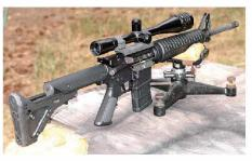
To wring out what the ArmaLite with the Geissele Match trigger and UBR stock would do, we stuck on our target Weaver 36X scope. The rifle averaged 0.7-inch groups at 100 yards. The stock was dead solid, yet collapsible. This was a solid, precise setup.
