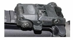
The rear sight can be kept out of the way if you have a scope or other unit on the rifle, yet opens to a touch. It locks up or down.
