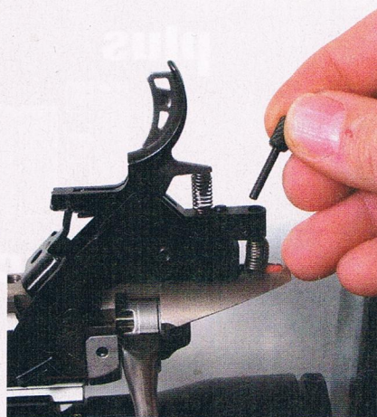
The excellent Savage AccuTrigger, like a Timney trigger, is fully adjustable.
