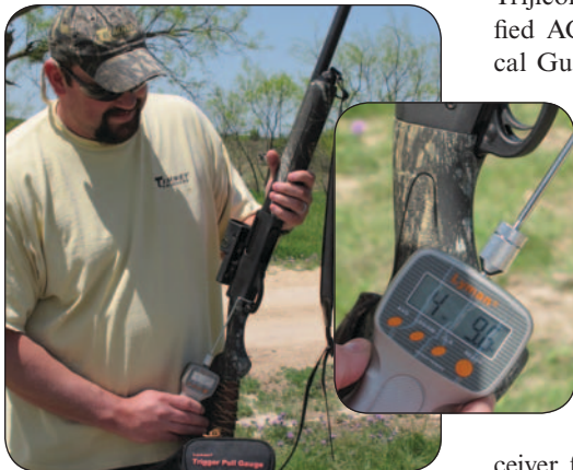
Chris Ellis of Timney measured trigger pull before and after installing the 870 Trigger Fix. The replacement on this gun was set to break at 3 pounds.
