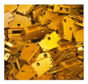
and disconnectors are from A-2 steel. All steel AR parts are through-hardened to a Rockwell hardness of 60.
