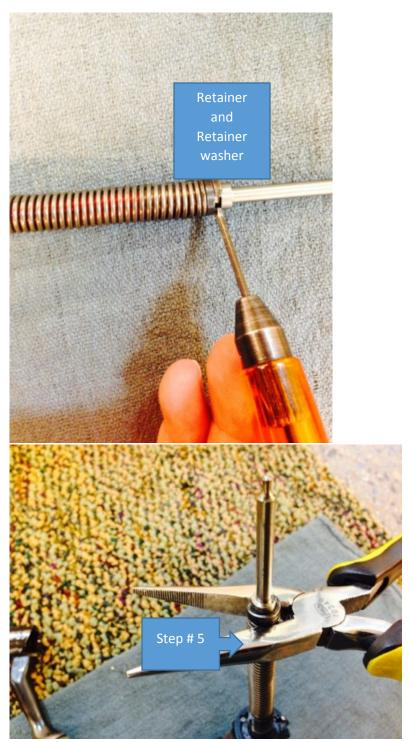
Pliers are between retainer and retainer washer, so that retainer can be removed.
