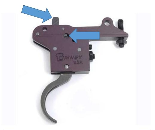
If you look through the window the lower arrow is point in when you engage the safety do the trigger and sear disengage? Mean is the sear lifted off the safety? You should be able to see it in the hole when you pull the safety back onto safe.
